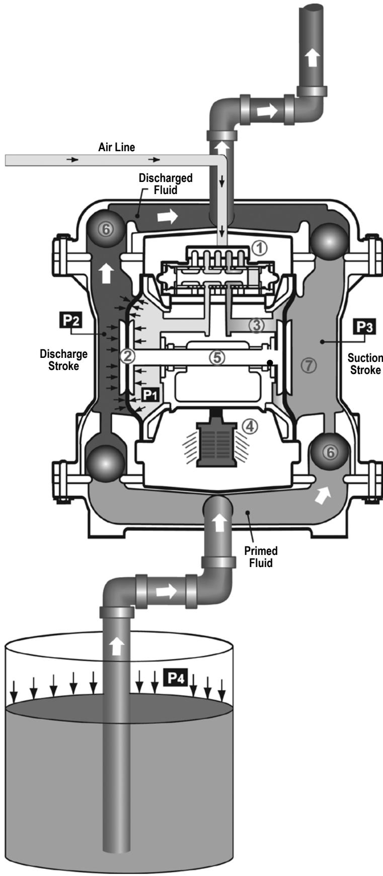
Air-Operated Double Diaphragm (AODD) pumps are powered by compressed air or nitrogen.
